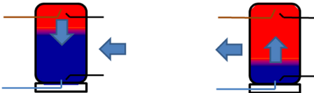
a) Charging phase of a charging storage system b) Discharging phase of a charging storage system
