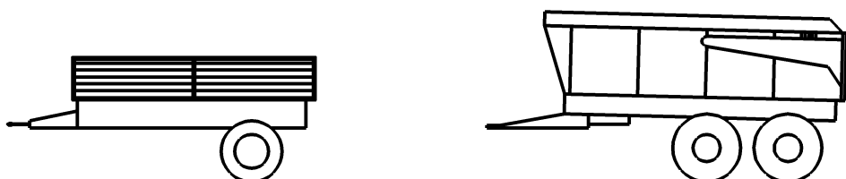
Figure 2 — Examples of semi-mounted trailer
