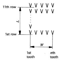
**3.3** coarseness of cut for files : Number of teeth of the principal cut per centimetre along the centre line of the file.
