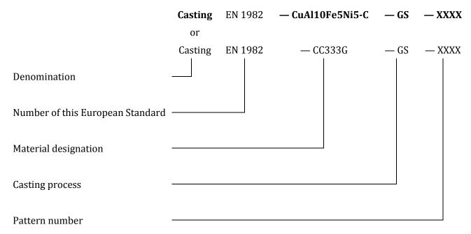
Ingots conforming to this standard, in material designated either CuAl10Fe5Ni5-B or CB333G, shall be designated as follows: I Ten STANDARD PREVIEW
