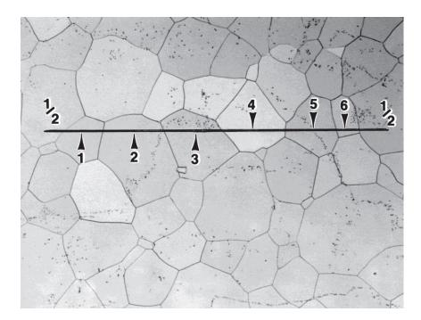
Interception, *N*, counts for a straight line on a single-phase grain structure where the arrows point to six intercepts and two line segments ending within grain  $(2 \times 1/2 = 1 N)$  and N = 7
