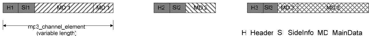
Figure 2 — Converting an MPEG-1/2 Layer 3 bitstream into mp3_channel_elements
