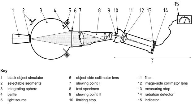
а The measurement and evaluation unit consists of the limiting stop, filter, image-side collimator lens, measuring stop, radiation detector and indicator.
