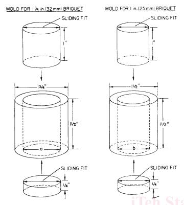
Note 1—Material: cold rolled or stainless steel. Dimensions a and b (inside diameters) are nominally 32 mm (11/4 in.) and 25 mm (1 in.). If an automatic polishing attachment is to be used, these dimensions should be specified to yield a briquet fitting snugly in the briquet holder.
