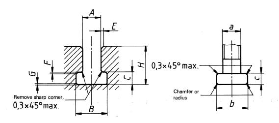
E, F and G: 45°-chamfer height or radius
