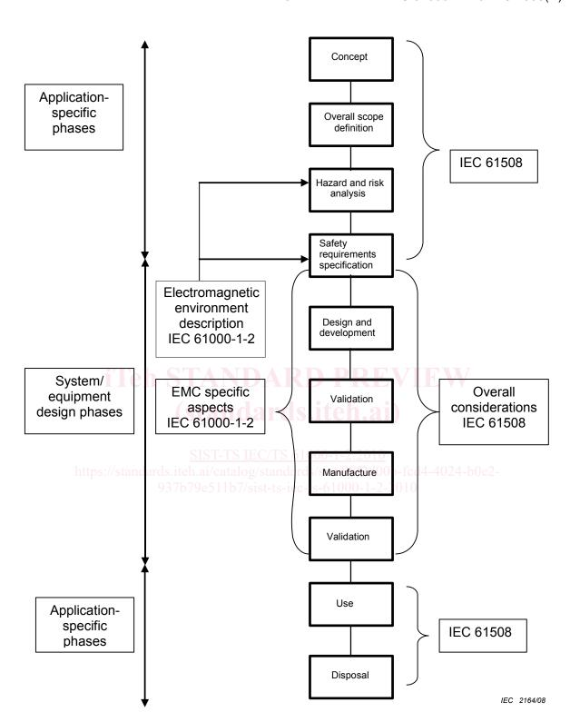
NOTE 1 The diagram shows a simplified overview of the relationship between IEC 61508 and IEC 61000-1-2. It should be noted that EMC issues may need careful consideration during lifecycle stages other than those covered by IEC 61000-1-2, e.g. maintenance activities for EMC characteristics may be required during the "use-of-equipment" phase to ensure continued safety-related system performance.
