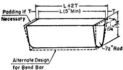
Note: Radius at Casting Coupon Interface at Option of Foundry
