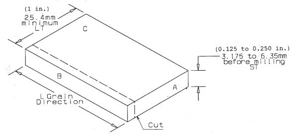
Face A is polished to .812  $\mu m (32 \ \mu in.) R_{a}$  or finer
