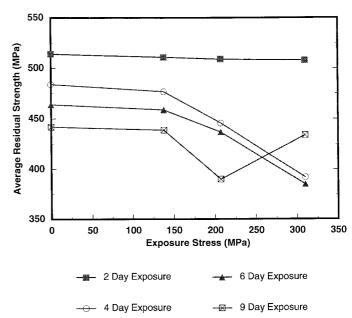
Note 1—Some specimens in this set did fail before the end of their scheduled exposure periods, but these failed specimens have not been included in the averages. The averages represent only specimens that survived to be tensile tested. The upturn in the nine-day data at 310 MPa is caused by not including failed specimens.
