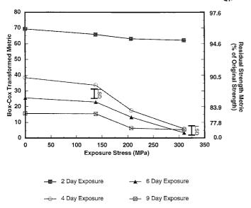
Note 1—In this case random values have been imputed for the failed specimens. Note the non-linear nature of the Box-Cox Metric (left Y-axis) as compared to the original metric (right Y-axis).
