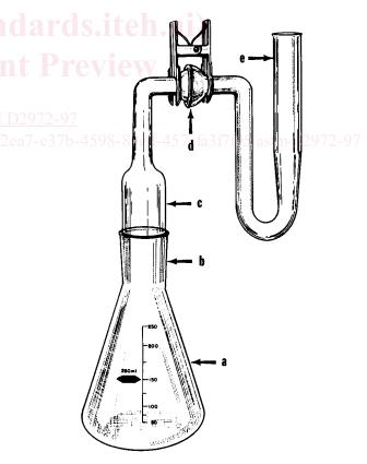
a) Generator flask, borosilicate glass, 250-mL capacity.
