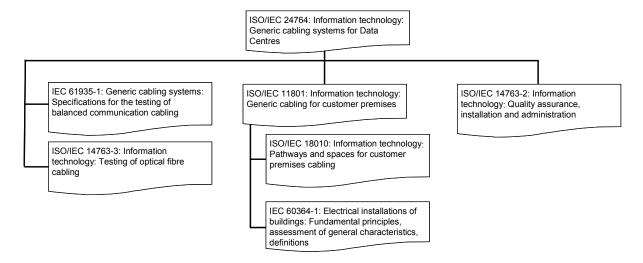
Scheme of the relationship between cabling standards such as ISO/IEC 11801 and other standards relevant for information technology cabling systems.
