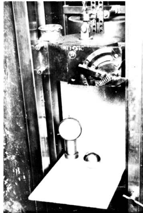
FIG. 5 Apparatus for Falling-Ball Indentation Test for Wood or Wood-Base Finish Flooring
