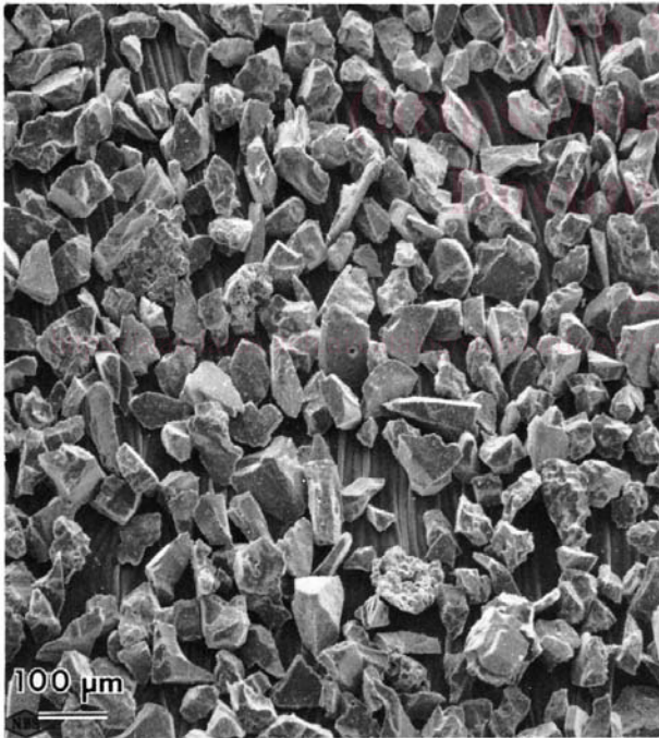
FIG. 3 Photomicrograph of 50 μm Al 2 O 3 Particles Used in Interlaboratory Testing
