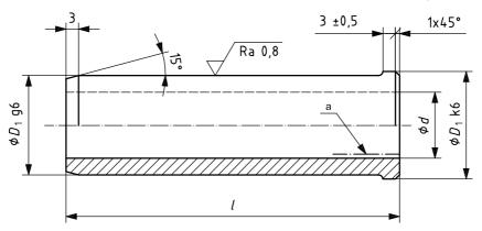
NOTE The centring sleeves are intended to fit in bores having a tolerance H7.
