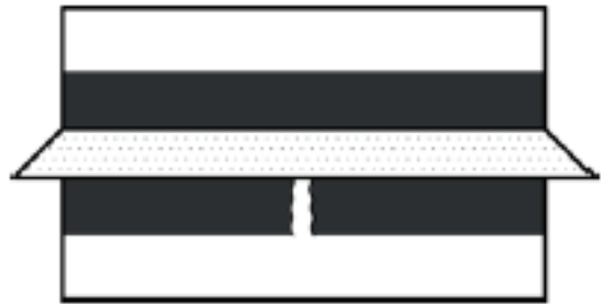
Stress Relief (for asphalt interlayer)
