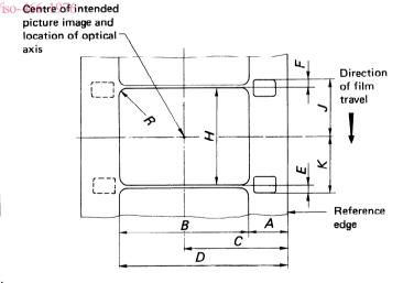
The film is shown as seen from inside the camera looking toward the lens with the photographic layer away from the observer.
