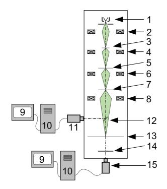
The digital camera (image sensor) position is different from the photographic film/imaging plate position.
