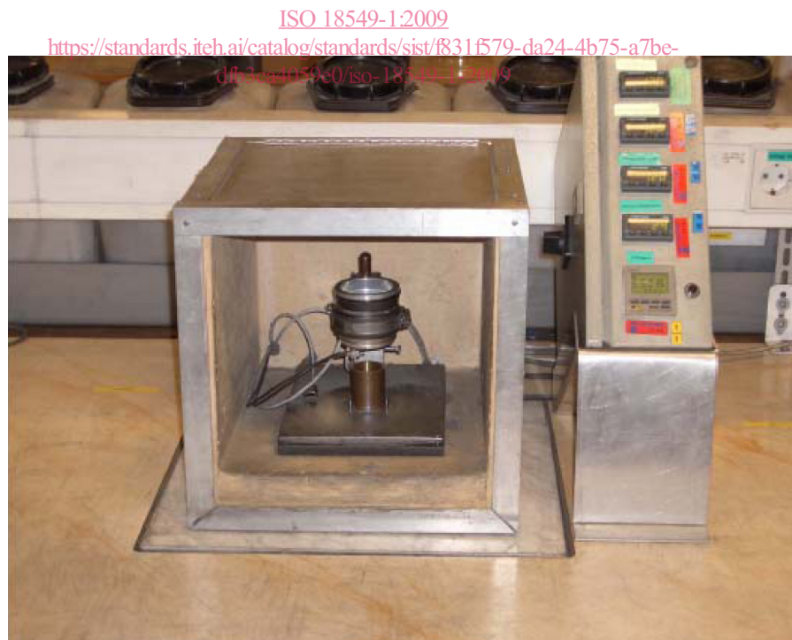
Figure 3 — Arrangement of the stand with funnel and cup, including heating devices
