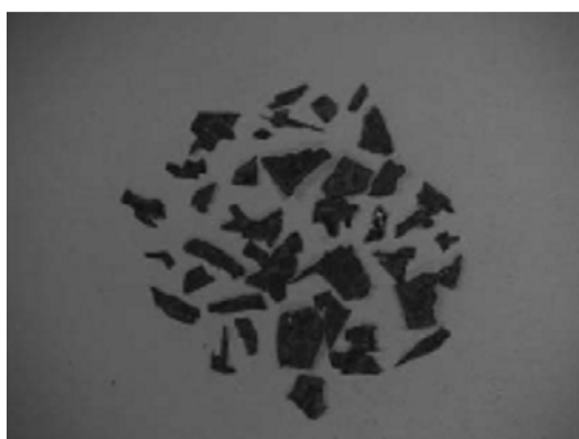
Figure 2 — Example of crushed UD CFRP fragments, which are approximated to rectangular shape shown by the line for the method C.
