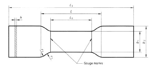
$b_1$  Width of narrow parallel-sided portion: 25,4 mm  $\pm$  0,1 mm
