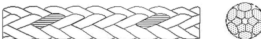
Figure 4 — Shape of a 12-strand braided rope (type T)
