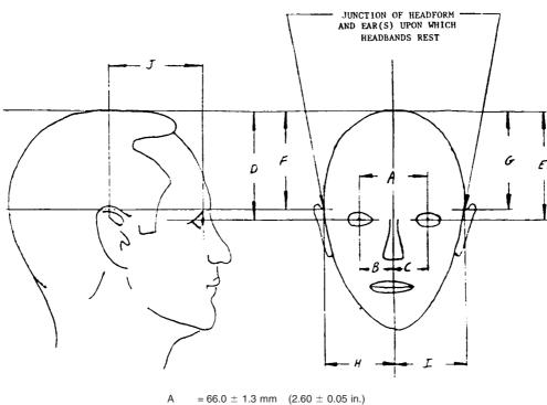
$\begin{array}{ll} A &= 66.0 \pm 1.3 \text{ mm} & (2.60 \pm 0.05 \text{ in.}) \\ B = C = 31.8 \pm 0.8 \text{ mm} & (1.25 \pm 0.03 \text{ in.}) \\ D = E = 109.2 \pm 2.5 \text{ mm} & (4.30 \pm 0.10 \text{ in.}) \\ F = G = 102.9 \pm 2.5 \text{ mm} & (4.05 \pm 0.10 \text{ in.}) \\ H = I = 78.7 \pm 2.5 \text{ mm} & (3.10 \pm 0.10 \text{ in.}) \\ J &= 82.6 \pm 1.3 \text{ mm} & (3.25 \pm 0.05 \text{ in.}) \end{array}$
