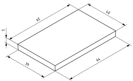
NOTE Dimensional tolerance shall be  $\pm$  1 mm.
