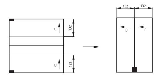
Figure 3 — Specimen preparation by cutting of tiles
