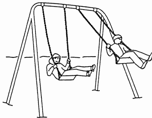
Figure 1: Example of swing with one rotational axis (Type 1)
