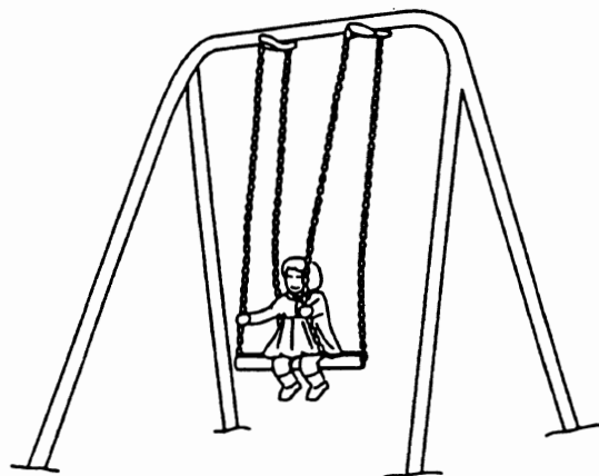
Figure 2: Example of swing with several rotational axes (Type 2)
