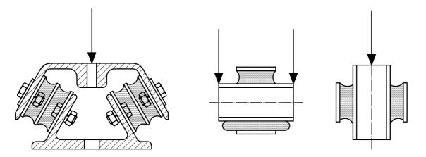
NOTE 1 When a resilient support has no parallel flanges, an auxiliary fixture should be included as part of the test element to arrange for parallel flanges.
