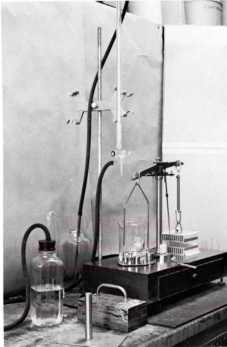
FIG. 1 Balance Modification with Buret Assembly
