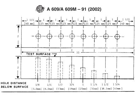
Note 1-Entrant surface shall be 250 µin. [6.3 µm] or finer.
