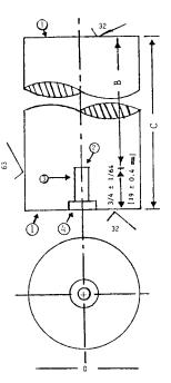
NOTE 1—Opposite ends of reference block shall be flat and parallel within 0.001 in. [0.025 mm].
