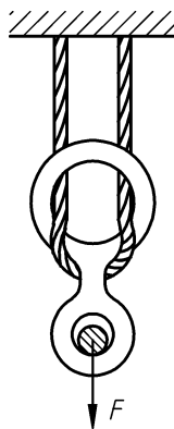
Figure 3 — Arrangement for testing the attachment opening
