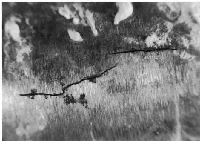
FIG. 2 Typical External Stress Corrosion Cracks (5× Magnification)
