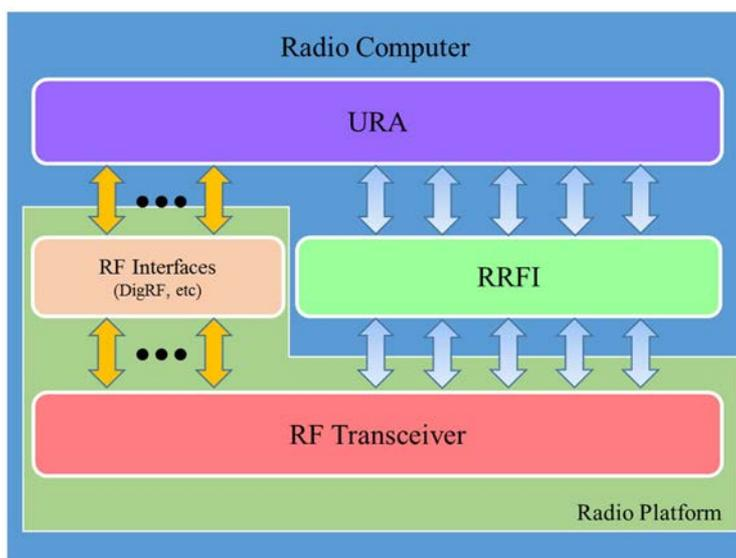
**Figure 5.1: Interconnection between URA and RF Transceiver using RRFI for reconfigurable MD**
