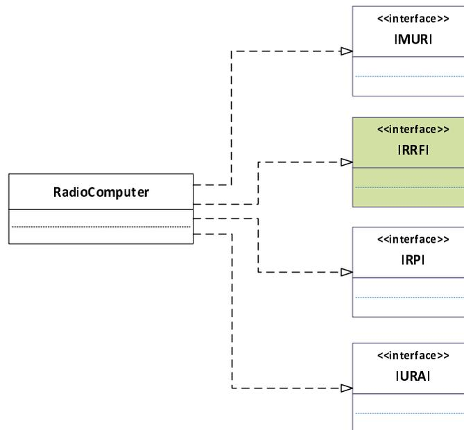
**Figure 4.2: UML class diagram for RC interfaces**
