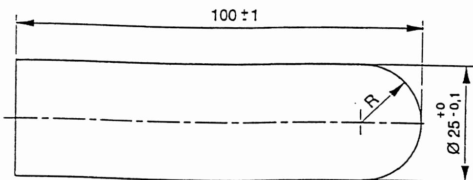
**Figure D.8: Finger rods**
