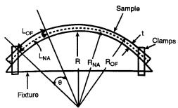
R = radius of jig  $R_{NA}$  = radius of neutral axis  $R_{OF}$  = radius of outer fiber t = thickness of specimen  $\theta$  = arbitrary angle  $L_{OF}$  = length of outer fiber  $L_{NA}$  = length of neutral axi
