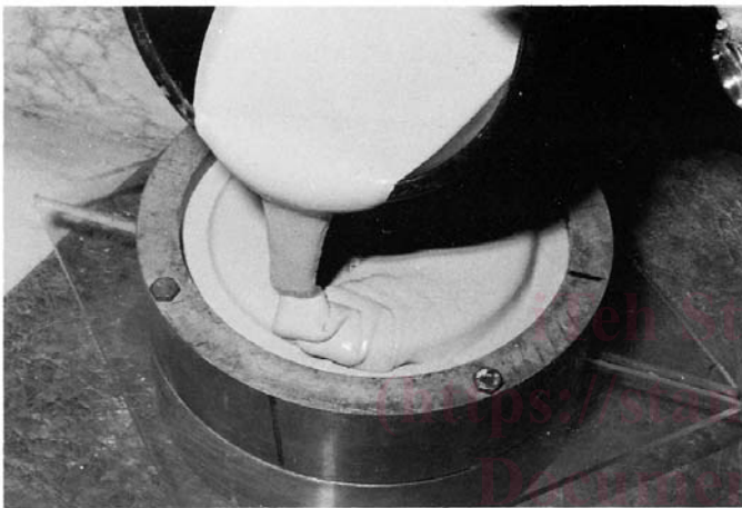
NOTE 1—Note the split plastic plates for isolating the shear zone. FIG. 3 View Showing Pouring Encapsulating Material Around Upper Half of Specimen
