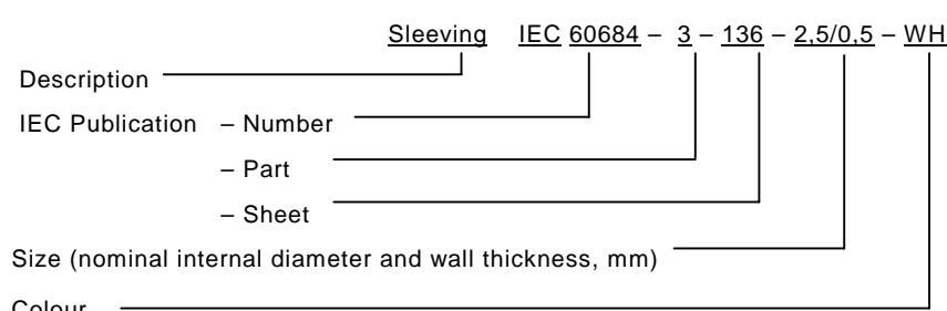
Any abbreviation used for colour shall comply with IEC 60757 where applicable. Non-standard colours shall be written out in full.
