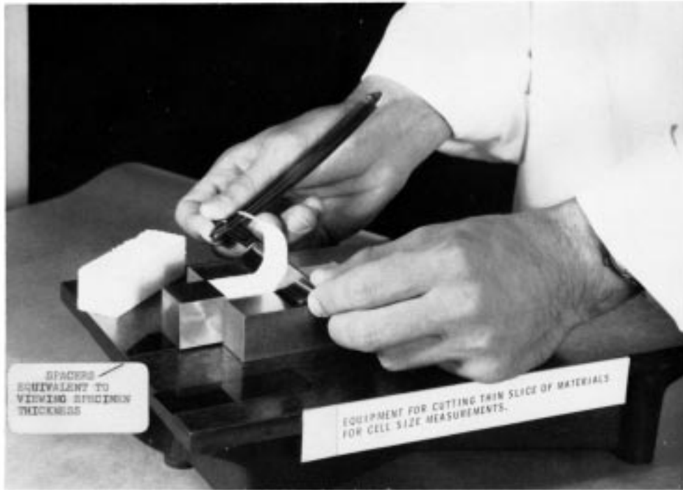
FIG. 1 Razor Blade Cell Size Specimen Slicer
