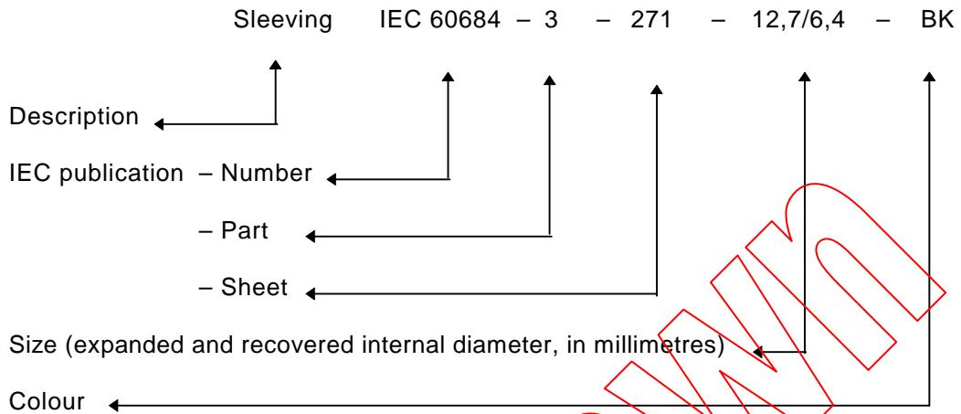
Any abbreviation for colour shall comply with IEC 60757, where applicable. Non-standard colours shall be written out in full.
