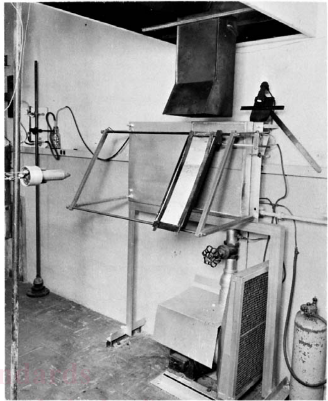
FIG. 1 Radiant Panel Flame Spread Test Equipment
