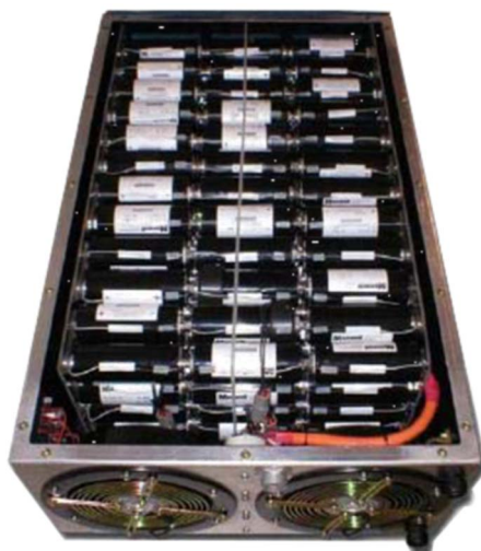
Figure 1: Example of a supercapacitor bank, 360 VDC - 150 kW 320 Wh
