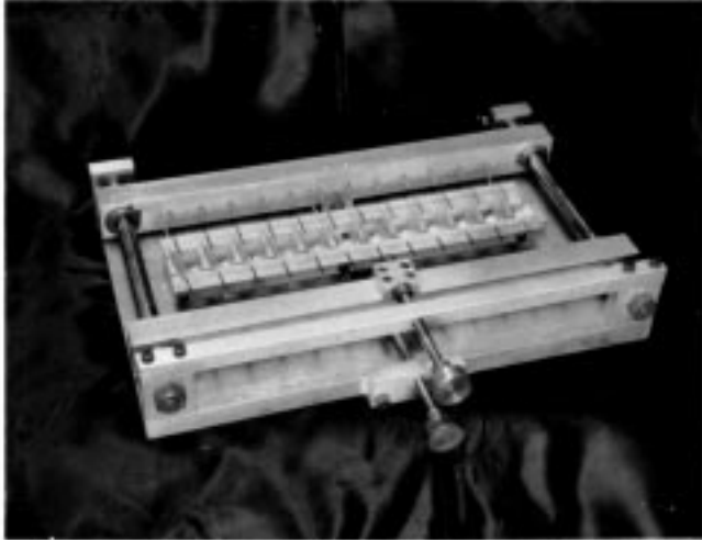
FIG. 3 Needle Insertion Jig
