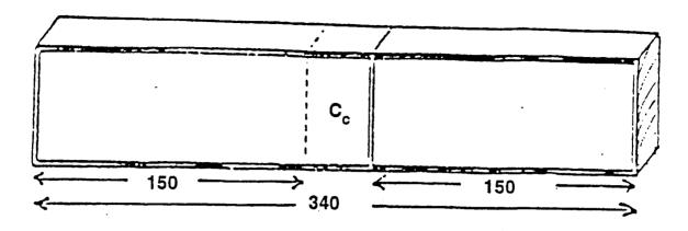
Figure 1: Cutting of the test panels
