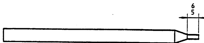
Figure 2 - Schematic view of pencil after sharpening
