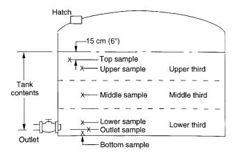
NOTE 1—The location shown for the outlet sample applies only to tanks with side outlets. It does not apply when the outlet comes from the floor of the tank or turns down into a sump. Bottom sample location must be specified.
