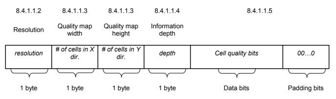
The first byte of the zonal quality data shall contain the resolution of the quality map in cells per decimetre. The next two bytes shall contain the number of cells in the quality map in the X and Y directions. The fourth byte gives the bit depth used for each cell. These header bytes shall be followed by the quality indication for each cell.
