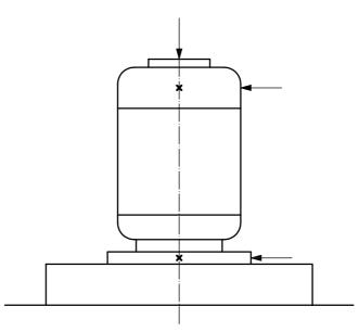
NOTE Measurements to be made at the bearing housing or, if not accessible, then at positions as close as possible to the bearing housings which provide adequate sensitivity to the machine dynamic forces.
