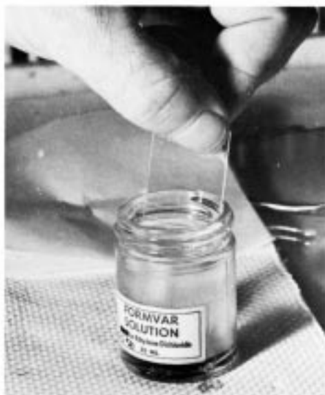
(a) Dipping Slide in Poly (Vinyl Formal) Solution
