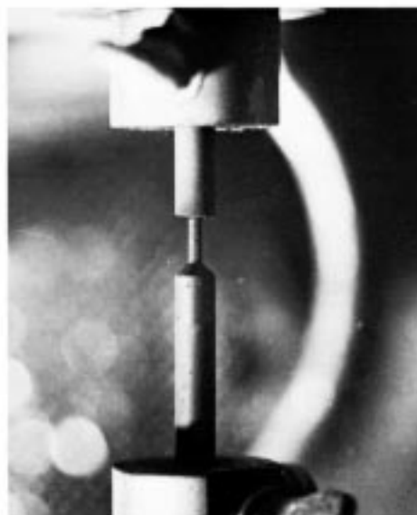
(b) Pared-Down Carbon Rod Tip for Evaporator
